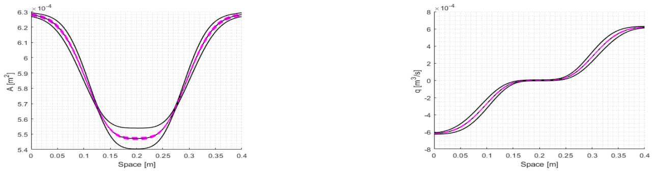
Figure 29: Test 2 with MUSCL-Hancock scheme. Average and average plus and minus twice the standard deviation (black line) for cross-sectional area A (left) and flow q (right). Four samples in magenta dashed line. M = 500 cells and \Gamma = 1 \text{ Pa m s} .
