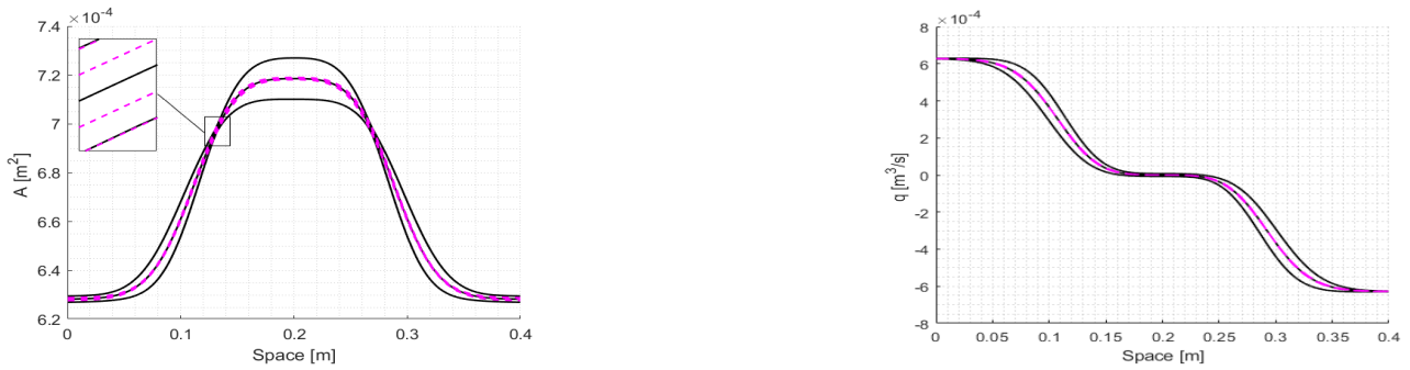
Figure 30: Test 3 with MUSCL-Hancock scheme. Average and average plus and minus twice the standard deviation (black line) for cross-sectional area A (left) and flow q (right). Four samples in magenta dashed line. M = 500 cells and \Gamma = 1 \text{ Pa m s} .
