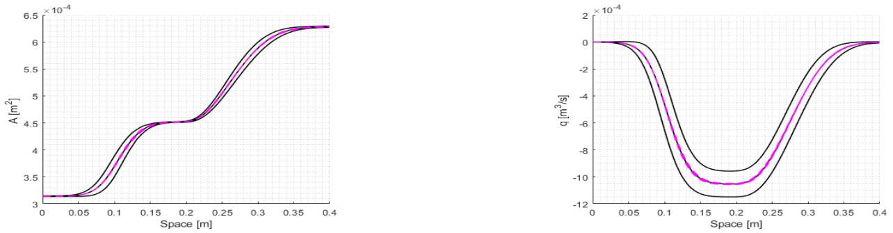
Figure 28: Test 1 with MUSCL-Hancock scheme. Average and average plus and minus twice the standard deviation in black line for cross-sectional area A (left) and flow q (right). Four samples in magenta dashed line. M = 500 cells and \Gamma = 1 \text{ Pa m s} .
